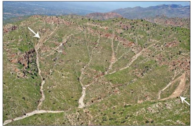
**Figure 5.** Hillslope failures of various sizes developed into debris flows in Soldier Canyon. Most failures initiated in small channels on hillslopes, but arrows point to large areas of hillslope colluvium failure. Photo provided by R.H. Webb.
