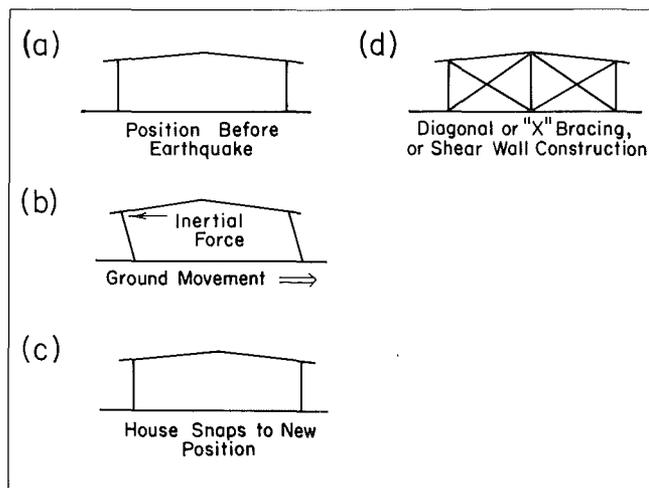
Figure 4. Dwelling damage in successive stages. (a) The original structure. (b) Ground motion with resulting inertial force in the opposite direction. (c) Second position of house. (d) Cross bracing of walls.
